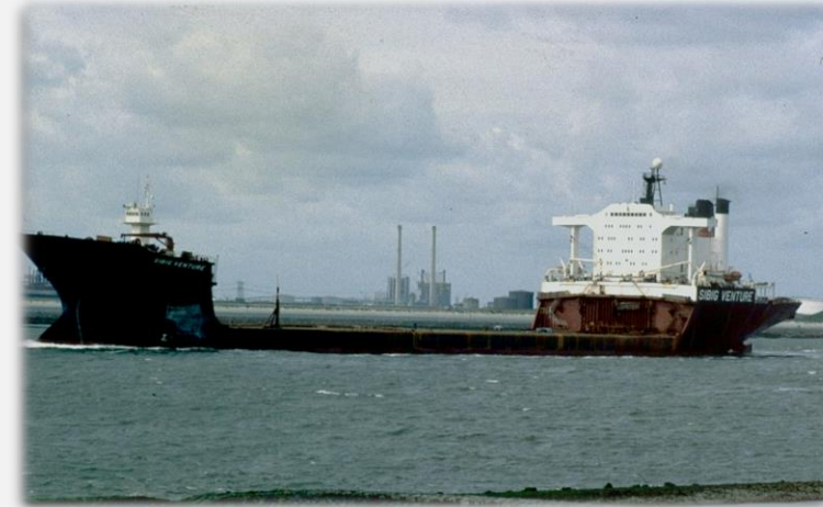
The dry tow heavy lift ship
